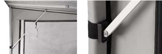
A foam with strap guarantees full sealing with the vehicle wall to avoid the wind from entering.
