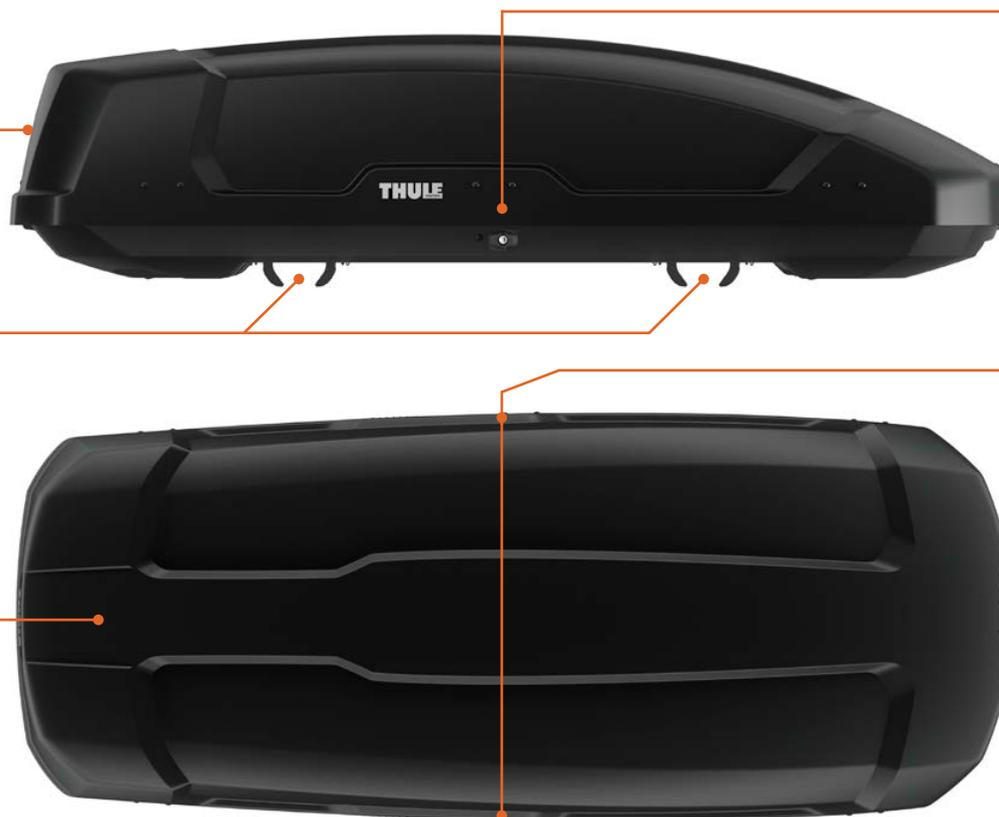
**Secured** - Comfortable to open and close thanks to the LockKnob that also helps to prevent damage to the Thule Comfort Key.
